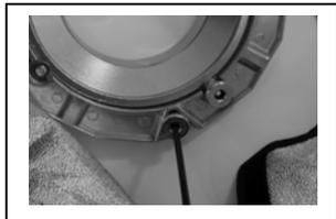
Now open up the rear end of the cover by pulling apart the Velcro fastening strips. This will give the necessary access to fit the speed ring. Next insert the rod with the ball end into the slot as shown opposite. Now insert the other 3 rods into the holes around the edge of the speed ring using every second hole from position of the first rod. After inserting the 3 straight rods, the rod with the ball end should be tensioned and locked in position.
