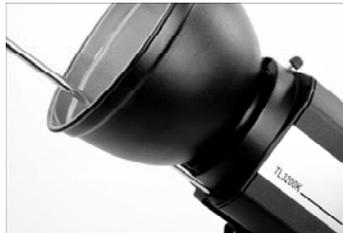
Push the umbrella shaft through the hole in the reflector and into the umbrella tube in the main body. Internal springs will grip the umbrella shaft. Adjust the shaft so that the light from the reflector fills the umbrella without spilling over the edges of the umbrella.
