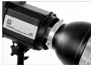
Pull back the spring locking lever as shown and rotate the reflector in an anti-clockwise direction until it is possible to pull the reflector away from the mount. To re-fit the reflector, insert the reflector into the mount ensuring that the hole for the umbrella shaft in the reflector is in line with the corresponding hole in the body. Push the reflector so that the locking lever moves backwards and turn the reflector in a clockwise direction, until it locks into place.
